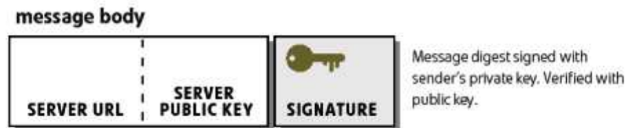
Figure 3: A certificate is made up of a server URL and a server public key
